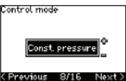
8. Select control mode i.e. Constant pressure
