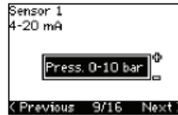
9. Select sensor range (see sensor nameplate)
