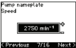
7. Enter motor nameplate RPM's (3450 for 60Hz motors)
