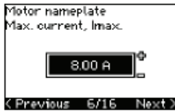
6. Select nameplate motor amps
